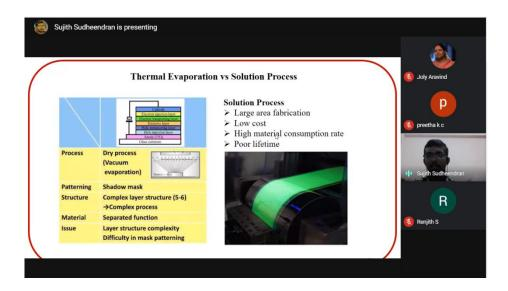
Comparison of thermal evaporation process and solution process in the preparation of OLEDs
