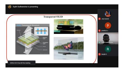
Transparent OLEDs have only transparent components (substrate, cathode and anode) and, when turned off, are up to 85 percent as transparent as their substrate. When a transparent OLED display is turned on, it allows light to pass in both directions. A transparent OLED display can be either active- or passive-matrix. This technology can be used for heads-up displays.
